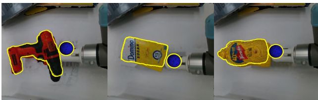
Fig. 7. Results of three example testing trajectory of the physical experiments. The predicted poses are obtained by applying the control forces from the initial pose and integrating forward in time. The predicted object poses with the optimized \theta highlighted with a yellow silhouette are overlaid with the ground-truth object and robot, and the background rendered from the optimized simulator. [Best viewed in color.]
