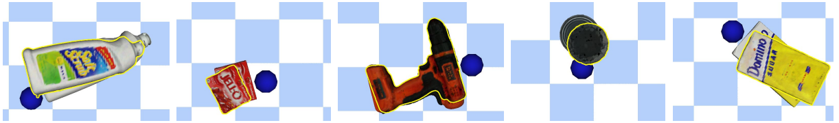
Fig. 5. The predicted and ground-truth poses of the 5 different objects at the end of sampled testing trajectories for the simulation experiments. After training, the predicted poses are obtained by applying the control forces from the initial pose and integrating forward in time. The predicted object poses are highlighted with a yellow silhouette and overlaid with the ground-truth object, blue floating spherical robot, and background. [Best viewed in color.]
